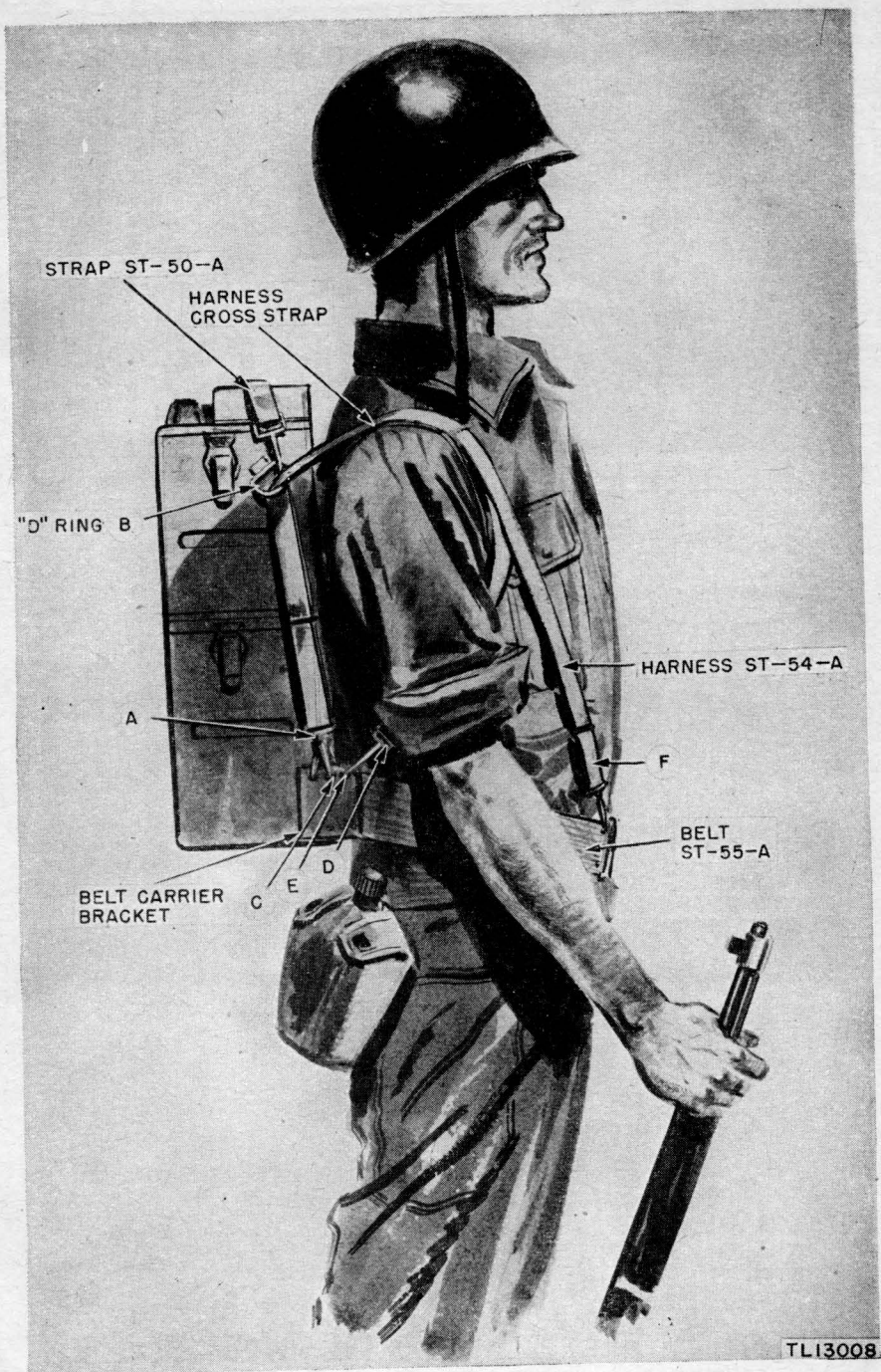
Figure 13. Radio Set SCR-300-A, Harness ST-54-A and Belt ST-55-A, installation detail.
