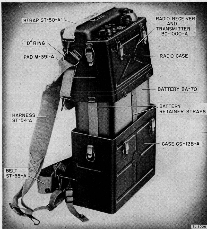
Figure 11. Radio Receiver and Transmitter BC-1000-A, radio set housing assembly after battery installation.
